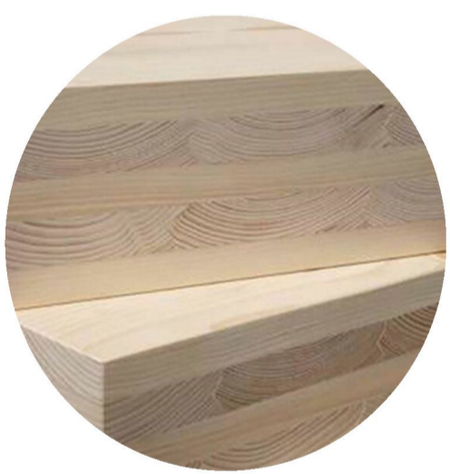
Cross Laminated Timber Glued together at 90°
